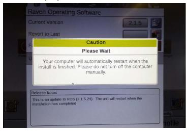
11. Remove the USB stick from the display while the screen below is displayed.
